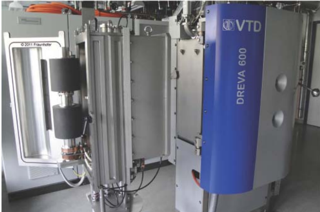
LaserArc® equipped industrial coating machine to deposit Diamor® coatings
