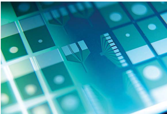
Silicon wafer with boron-doped diamond macro electrode chips and microarray sensor chips
